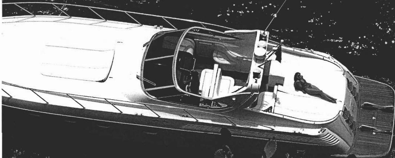
The self-draining cockpit, deep and long, extends on two levels: the lower, towards aft, is equipped with sofas, a sundeck, a wet bar that can be arranged also for hosting an additional fridge and a grill, a compartment for the raft and the door leading to the engine room. The upper-deck, able to comfortably accommodate up to seven people, houses a table and gives the possibility to the pilot to adjust his seat for sit-
